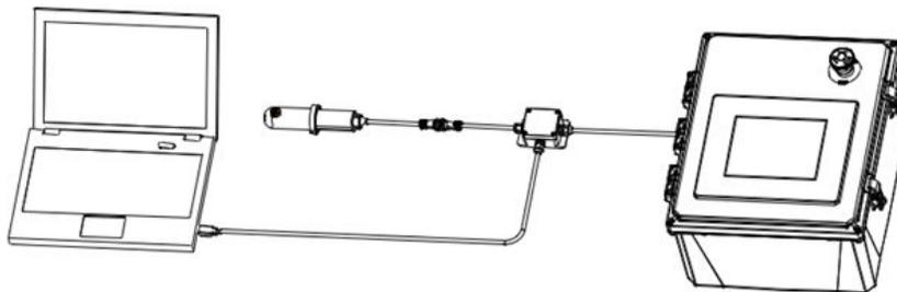
Figure 5. USB connection to ST-525 Series sensor
