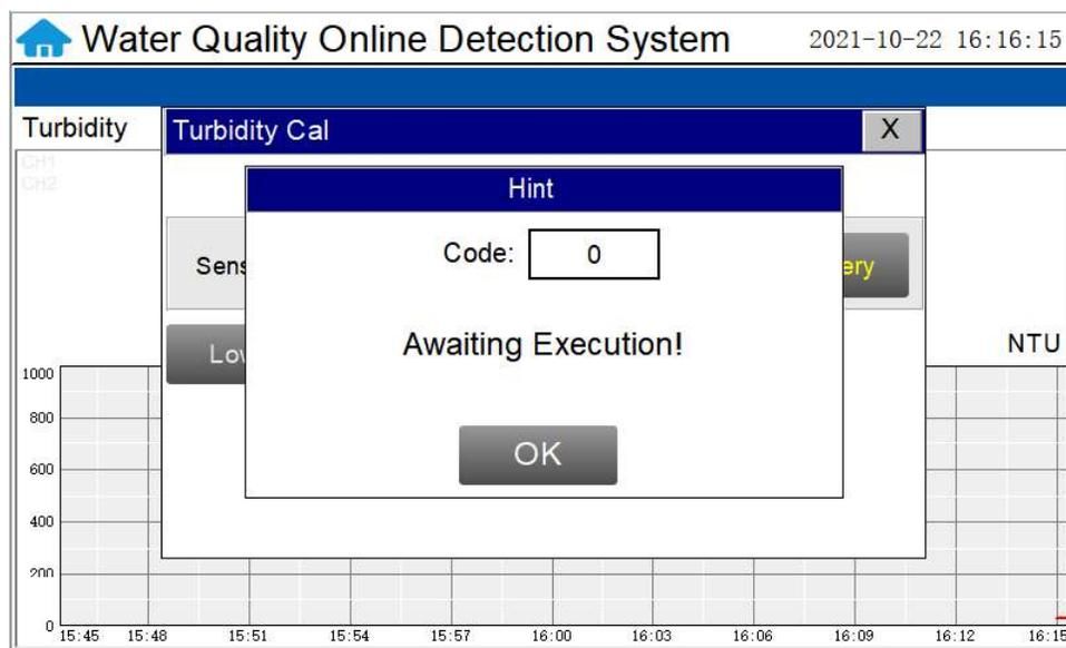
Figure. 19- Awaiting execution Screen of Turbidity Calibration
