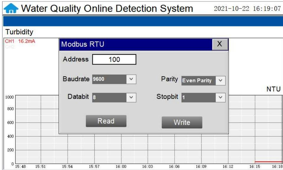
Figure. 14 - Modbus RTU Setting
