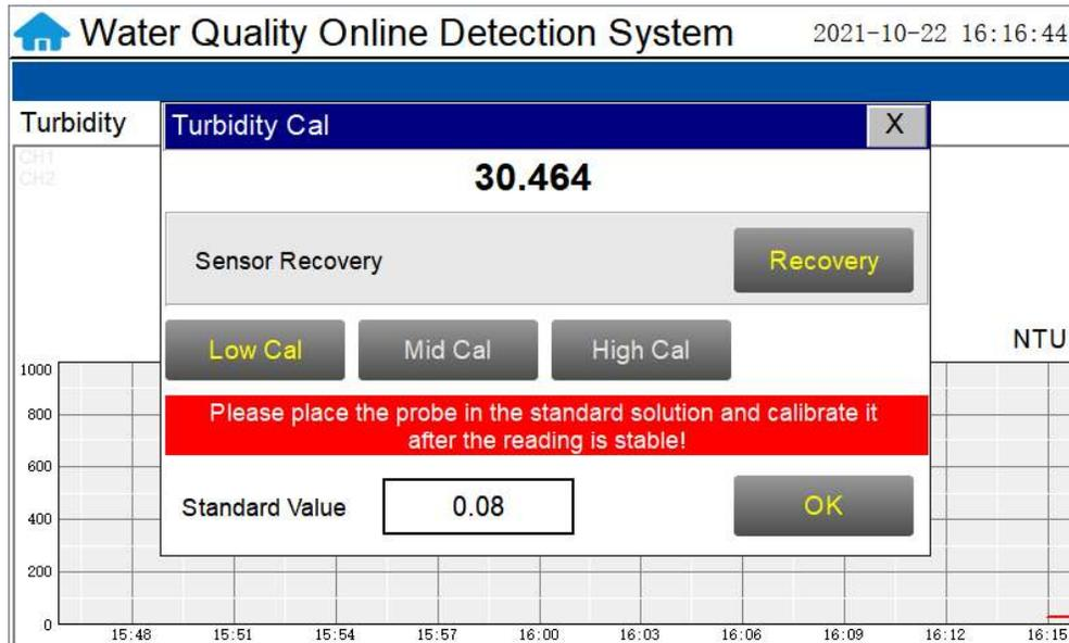
Figure. 18 - Enter the standard solution value
