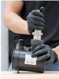
Tighten Sensor Nut
