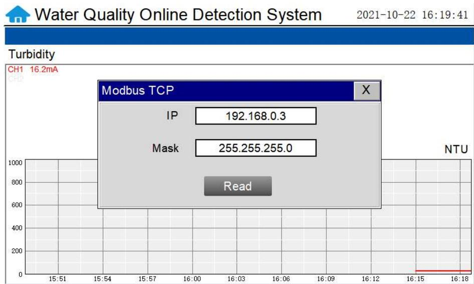
Figure. 15 Modbus TCP Setting
