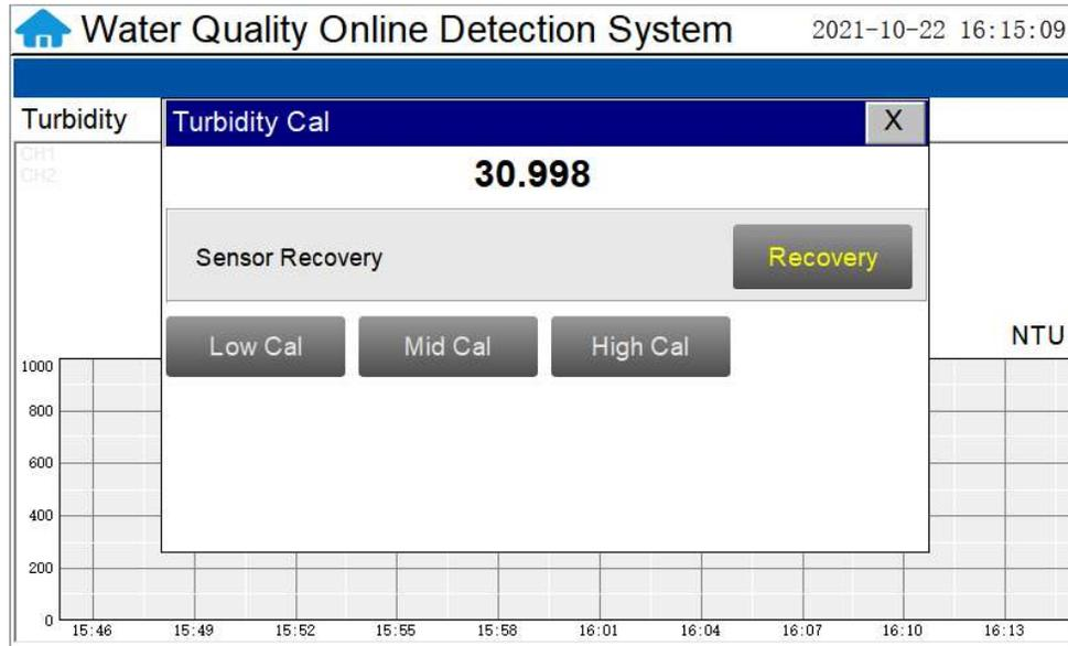
Figure. 17 - Turbidity Calibration Screen
