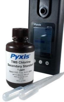
**Figure 24.** TMB Chlorine Secondary Standard 1 ppm
