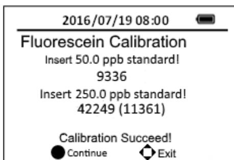
Figure 11. Middle Range Fluorescein Calibration
