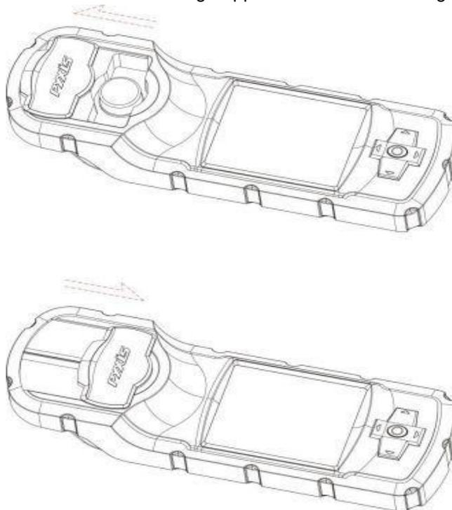
**Figure 3 Open and Close the Light Shield Cover**
