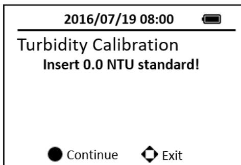
Figure 20. Turbidity Calibration-1
