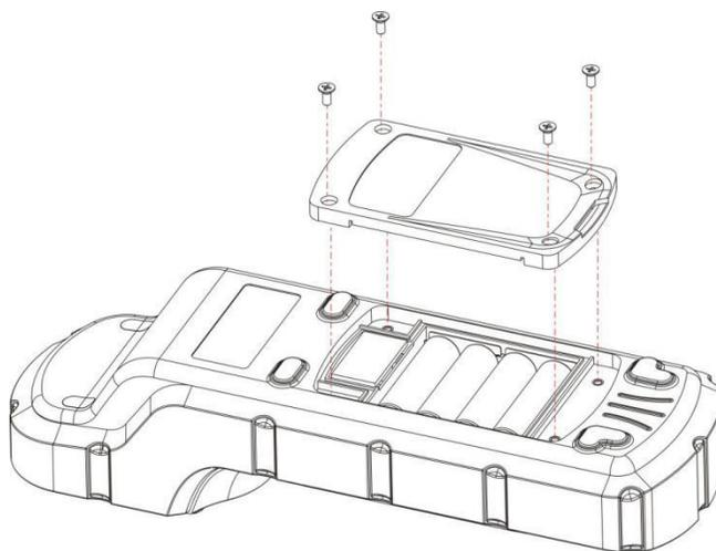
Figure 4 Replace Batteries
