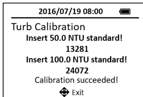
Figure 22. High Range Turbidity Calibration
